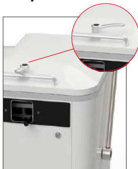
1. Lift the cover, releasing the hook
