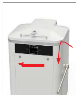
6. Bring the pressure handle forward until the dough is completely cut
