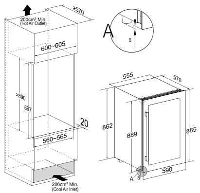
To fix the appliance with Cabinet, pls. screw the 3 screws (ST4.2\*12mm) through the Top Bracket. The Top Bracket is pre-installed on top of appliance.
