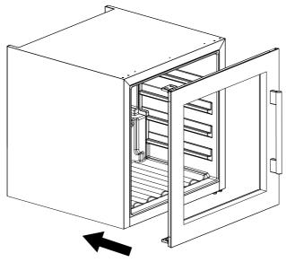
o Install the Upper Door Shaft (Left/Right) on the upper left door corner by screwing the 2 Phillips Flat Screws (M4\*8);
