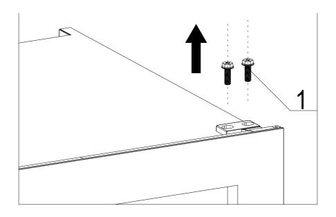
o Unscrew the 2 Phillips Flat Screws (M4\*8) from the right lower Door Hinge;
