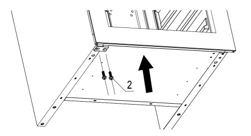
o Install the Top Bracket by screwing the 3 screws.
