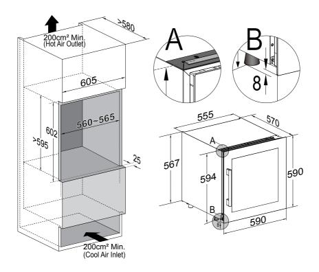
To fix the appliance with Cabinet, pls. screw the 3 screws (ST4.2\*12mm) through the Top Bracket. The Top Bracket is pre-installed on top of appliance.
