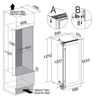
To fix the appliance with Cabinet, pls. screw the 3 screws (ST4.2\*12mm) through the Top Bracket. The Top Bracket is preinstalled on top of appliance.
