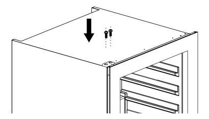
Install the Upper Door Shaft (Left/Right) on the upper left door corner by screwing the 2 Phillips Flat Screws (M4\*8);
