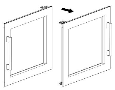
Make sure the hole position of the left door hinge is aligned with the hole position on the cabinet;
