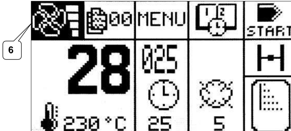
**Selecting the steam exhaust valve open or closed**
