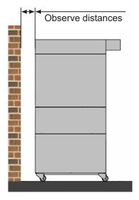
Electricity, water, waste water and exhaust connections are located on the back of the appliance/combined appliance. These must be accessible when required.
