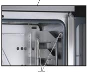
The support racks can be easily dismantled without the use of tools.
