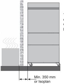
The appliance/combined appliance must be installed at a minimum distance of 350 mm from other heat sources (>80 °C). If the minimum distance cannot be achieved a heat shield (e.g. Isoplan) must be provided by the customer.
