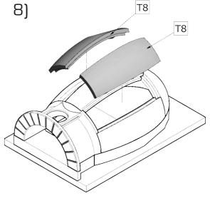
Place the last two shaped pieces into the remaining space so that the locks match.
