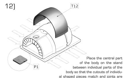
as narrow as possible. If it is necessary to align the parts, place the supplied dilatation pads under the side edges, preferably at places marked by arrows (9 points). Do not remove the pads. If you use more than 2 pieces of pads on top of each other, bind them together using silicone caulk.
