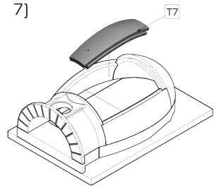
Place the central part of the arch with a hole towards the chimney. Shape should be placed on the top of the arch.
