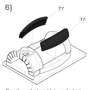
Place the small side arch between the front and rear arch. Side arches should be placed with a hole towards the front portal.
