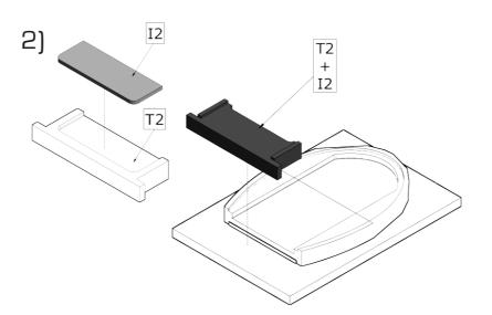
Using a bonding agent, glue the bio-mat (part I2 front bottom according to the cutting plan of the bio-mat) into the bottom cutout of the bottom front plate, place the plate by this bottom side with the bio-mat to the stand
