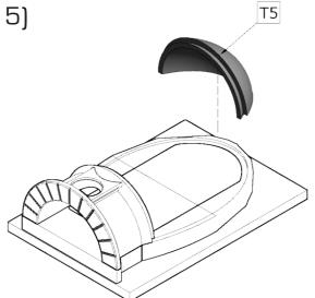
Place the rear arch on the rear plate of the bottom.
