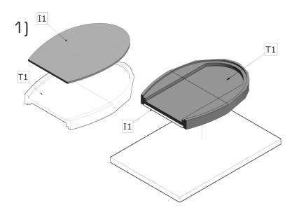
Using a bonding agent, glue the bio-mat (part I1 rear bottom according to the cutting plan of the bio-mat) to the bottom cutout of the bottom rear plate, place the plate by this bottom side with the bio-mat to a stand.
