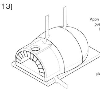
Apply silicone caulk between the body parts and along oven circumference between the bottom edge of the body and the stand - into the formed joint, the used dilatation pads should also get fixed.
