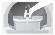
Pull the fluff filter out of the filter holder.
