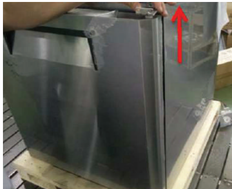
2) Remove the top hinge from the unit.
