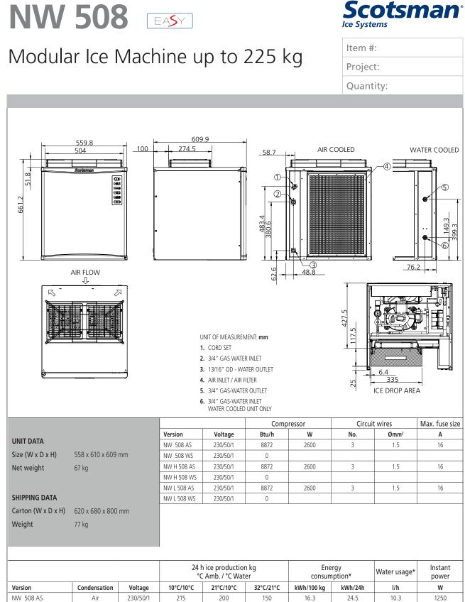
NW 508 WS Water 230/50/1 NW H 508 AS 230/50/1 225 205 155 14.8 22.9 10.1 Air NW H 508 WS 230/50/1 Water NW L 508 AS 230/50/1 210 200 145 15.9 23.0 9.7 Air NW L 508 WS 230/50/1 Water
